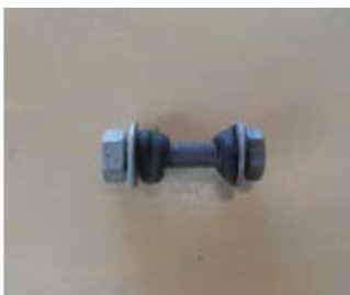
Representation of the nut and bolt arrangement with the arboseal wrapped around under the washers
