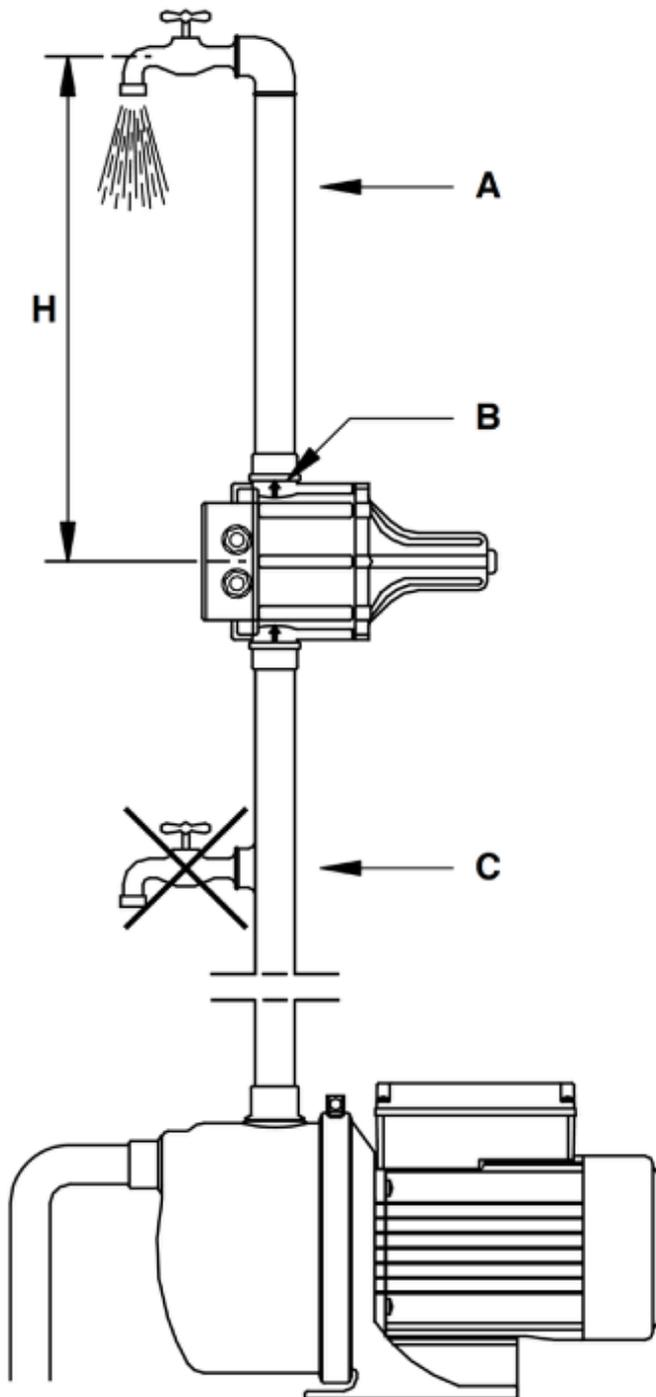
The unit can be fitted directly to the discharge port of the pump or between the pump and the first draw-off point.
