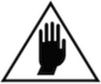
In the 'HAND' position the pump(s) controlled by the switch will normally run at full speed and completely independently of any control devices, and can result in pump(s) running against a closed valve head if there is no draw.
