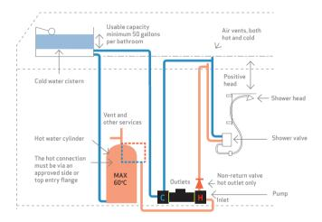
Right Pump twin ended positive head with up and over pipework and natural flow of 1 Litre/min per side.
