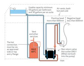
Negative head When the distance between the cold water storage cistern and the shower head is 600 mm or less, or when the natural flow is poor or less than 2 litres per minute of combined hot and cold it is possible a negative head pump may be required.
