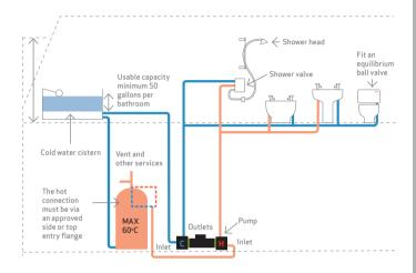
Right Pump twin ended universal to a bathroom in a loft conversion.
