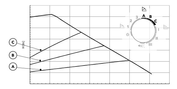
Proportional pressure functional mode is recommended in systems with relatively large pressure losses in the distribution pipes such as **radiator heating loops**.
