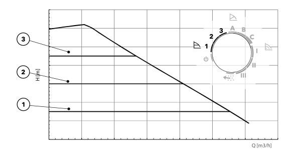
Constant pressure control is ideal for systems in which the distribution pipe is non-existent or very short. A prime example is **underfloor heating**. The distribution pipe consists in most cases of an extremely short pipe run and the manifold. In such cases, system resistance is negligible.
